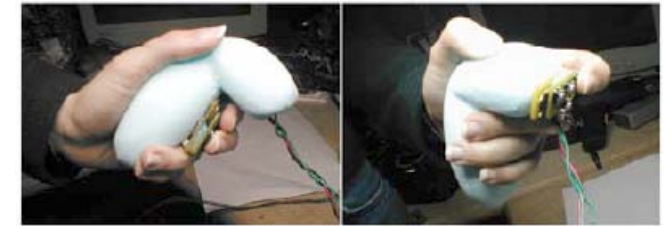
Figure 2. Wireless knob and buttons used within a foam model of a concept game controller.
