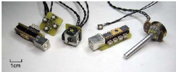
Figure 6. Wired components. (left to right) I/O Breadboard component, 4-button array, analog joystick, D/A Input Component, single button, and analog knob.
