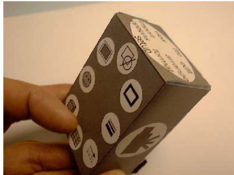
Figure 8: A ToolStone device with labels on each face. A (novice) user would be able to visually inspect available commands by physically turning the device.
