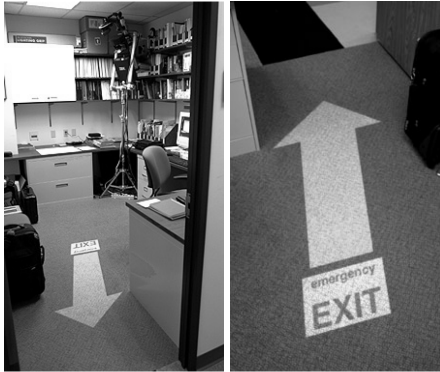
Plate 7 Fig. 1. Navigation application of an everywhere displays projector: pointing to the emergency exit.
