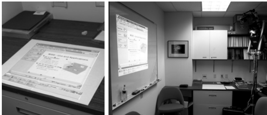
Plate 7 Fig. 2. An everywhere displays projector moving a desktop application from the top of a table to a whiteboard.
