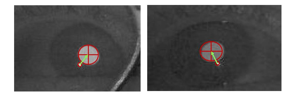
Measuring the direction and distance between glint and center of the pupil
