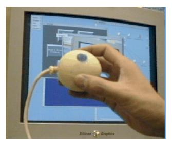
The form factor of devices has a significant impact on the pointing performance. E.g. Fingerball vs. glove
