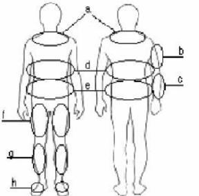
Fig. 1, The general areas we have found to be the most unobtrusive for wearable objects are: (a) collar area, (b) rear of the upper arm, (c) forearm, (d)rear, side, and front ribcage, (e) waist and hips, (f) thigh, (g) shin, and (h) top of the foot.
