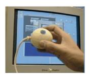
The form factor of devices has a significant impact on the pointing performance. E.g. Fingerball vs. glove
