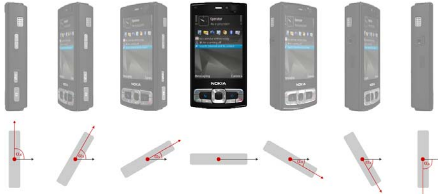
Figure 3. Rotation around the phone's x-axis. The bigger the angle, the faster the cursor moves to the left (left side) or right (right side). The center depicts the zero point (no movement).
