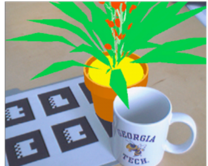
Figure 5: A screenshot of a running DART program. The "program" for this example is shown in Figure 4. There are two objects, the virtual flowerpot, and a "physical" cylinder that is aligned with the cup (hard-coded relative to the fiducial in this example) and used to cause the cup to interact correctly with the flowerpot.
