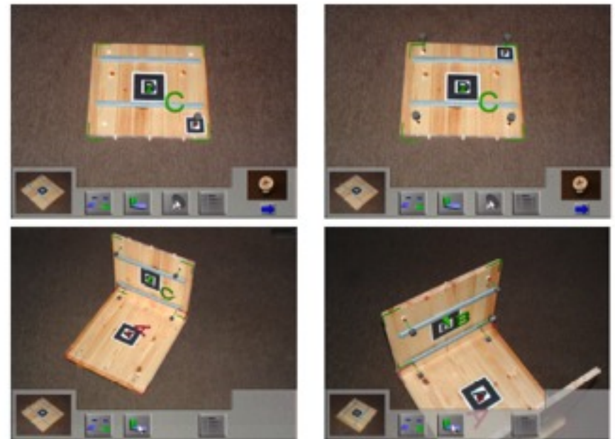
Figure 8. The expert assembles in a step-by-step approach the different parts. The undetectable and detectable elements are built together with the authoring wizard.
