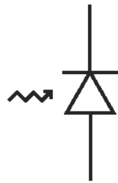
Modeled as capacitor in parallel with current source (photocurrent)
