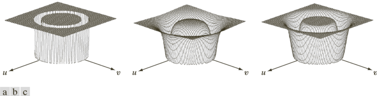
FIGURE 5.15 From left to right, perspective plots of ideal, Butterworth (of order 1), and Gaussian bandreject filters.
