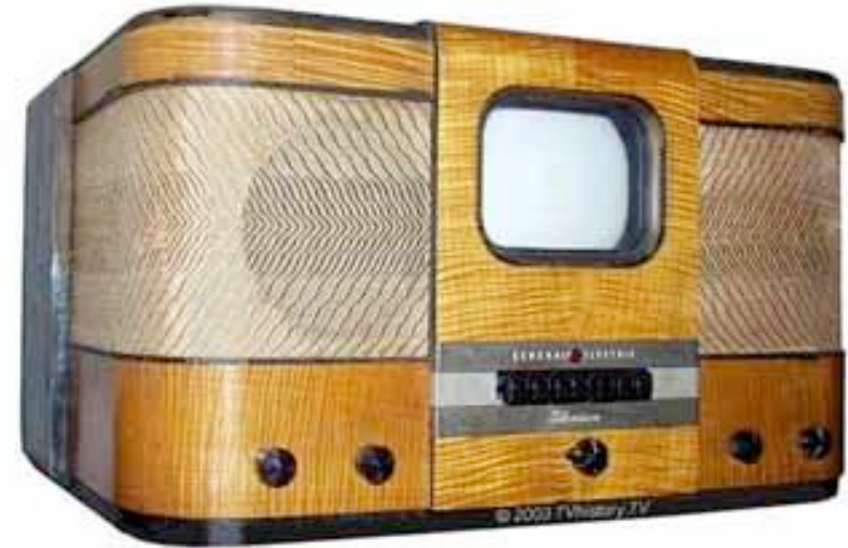
1938 General Electric (USA) 5" CRT - Tabletop Prototype 7 channels - with sound
