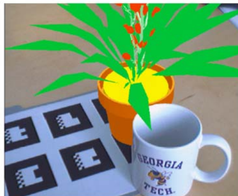
Figure 5: A screenshot of a running DART program. The "program" for this example is shown in Figure 4. There are two objects, the virtual flowerpot, and a "physical" cylinder that is aligned with the cup (hard-coded relative to the fiducial in this example) and used to cause the cup to interact correctly with the flowerpot.
