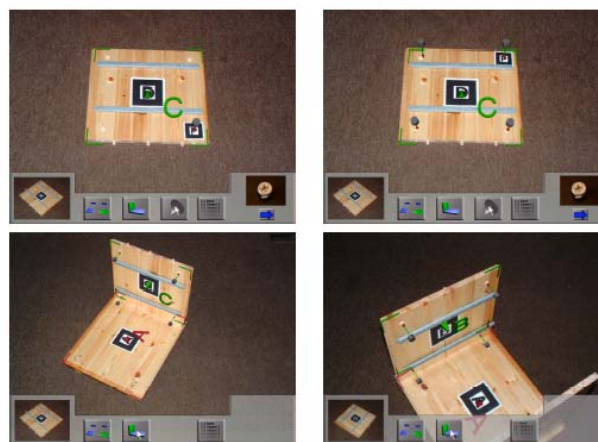
Figure 8. The expert assembles in a step-by-step approach the different parts. The undetectable and detectable elements are built together with the authoring wizard.
