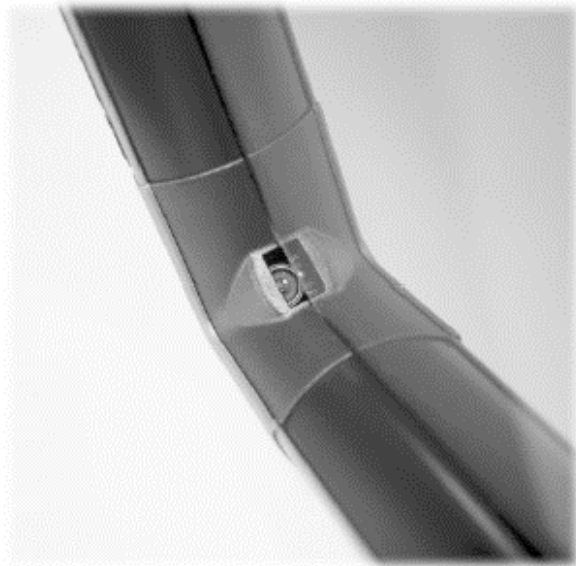
Figure 1: DViT Technology Camera
