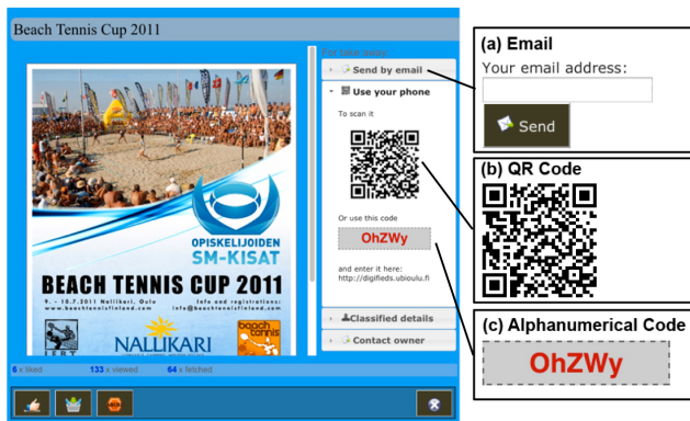
Figure 6. Taking away content: Users can send digifieds to their email address or transfer them to their mobile phone using either the QR code or the alphanumeric code.
