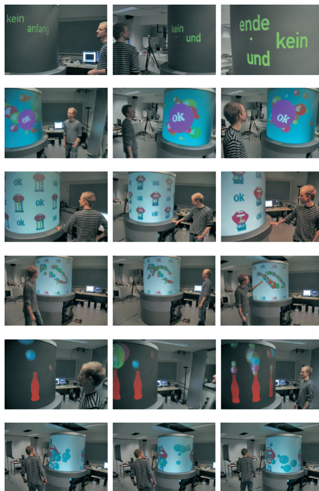
Figure 4: Developed applications for the cylindrical screen: (1) Reactive animated typography. (2) Direction of the viewer. (3) Tales around the column. (4) Movements of the viewer. (5) Reactive ambient column. (6) Interactive multi-player game (detailed descriptions below).
