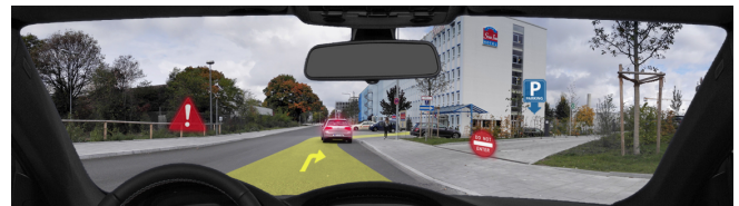
Figure 1. Full windshield display presenting world-fixed information
