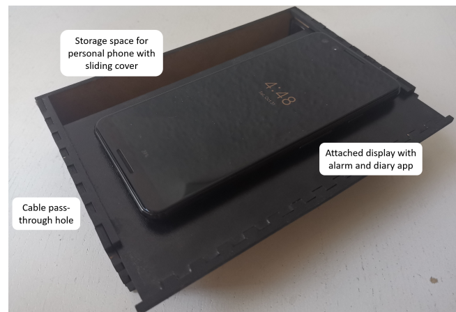
Figure 1: The proof-of-concept prototype, consisting of a laser cut box with a sliding cover, charging cable hole, and a display on top where users can set alarms.
