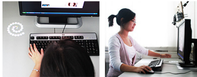
figure 4. A projector and a web cam are mounted over a desk for ambient projection and peripheral interaction.
