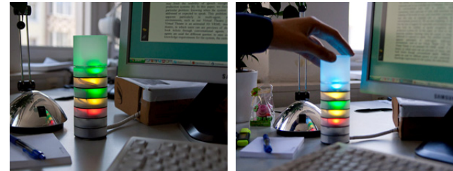
figure 5. A tangible representing presence information of the users and their colleagues. It also offers manipulation of one's status by turning and pushing down the top.
