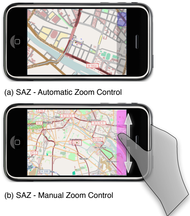
Figure 2: Placement and visualization of the zoom level slider in the SAZ map interface: (a) shows the SAZ interface in automatic zooming mode (no touch on slider), (b) shows the manual zooming mode (finger on slider thumb controls the zoom level).
