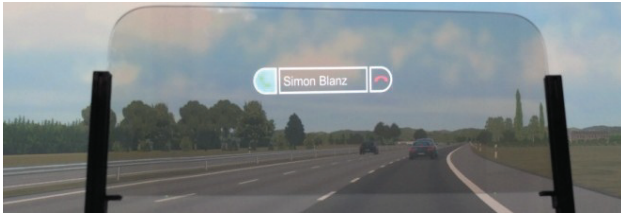
Figure 2: Visualization of the use case 'call' on the HUD in front of the driving scene from the driver's perspective.
