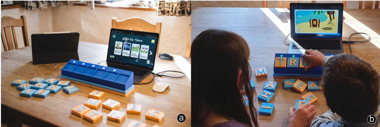
Figure 1: SpellBoard for children learning German spelling: a) The whole setup with 20 letter blocks, a board with six positions to put letter blocks, and a laptop for showing spelling tasks; b) Two children in our study were spelling “Truhe” (i.e., chest in English).
