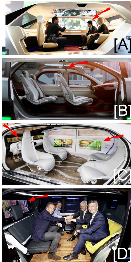
Figure 2: Examples of displays in interior concepts of automated vehicles. Red arrows indicate the position of attached screens. A [13], B [6], C [3], D [8]
