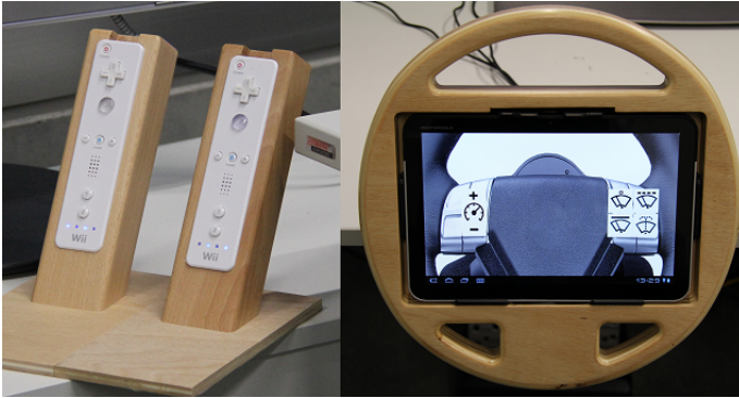
Figure 5.11: We used two WiiMote controllers and touch buttons on the steering wheel to replicate a traditional automotive interface for the traditional interaction condition.
