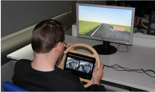
Figure 5.2: Study setup of the formative study. The scenarios were presented on a display that was mounted to the steering wheel. This speech-enabled multi-touch steering wheel allowed to record speech commands and touch gestures. For a more realistic environment, the experiment was conducted in a simple driving simulation.
