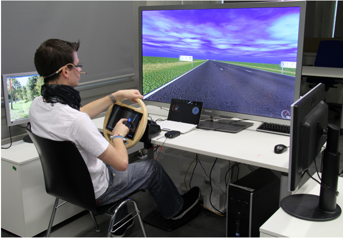
Figure 5.7: Setup of the prototype to evaluate the multimodal interaction style in a driving simulation: The participants use a customized steering wheel and pedals to drive in a driving simulator such as the LCT environment shown in this example. Additional screens around the driver simulate windows and external mirrors on the left/right side of the vehicle as well as the rear window and wiper (not shown here). The multitouch-enabled steering wheel allows for touch gesture input, and a microphone enables the use of speech commands.
