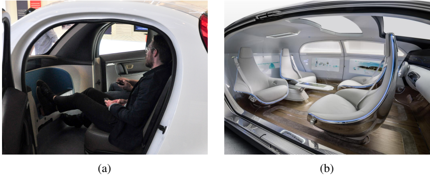
Figure 2.2: Exemplary concepts for the interior of automated cars: (a) The envisioned automated car by Google only has an emergency-off button as major interface element but no controls to manually drive the car. (b) The prototypical Mercedes F 015 is able to drive automated but also provides a steering wheel for manual driving. Here, the configuration for automated driving is shown. Image sources: (a) Own image, (b) ©Daimler AG, used with permission.
