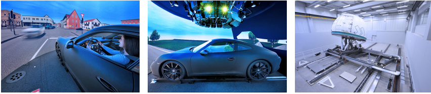
Figure 2.4: The Stuttgart Driving Simulator provides a 360 ° simulation dome that fits complete production vehicles. Mounted on a motion platform with 8 degrees of freedom, it allows to also perceive motion as it occurs when driving in the real world. Image source: ©FKFS, used with permission.
