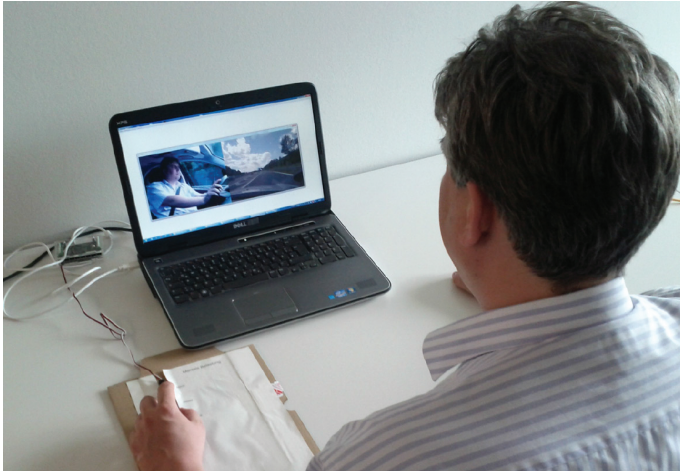
Figure 4.5: A participant is performing the post-hoc subjective video rating task. The participant watches a replay of his ride and continuously rates the perceived workload of the situation shown in the video.
