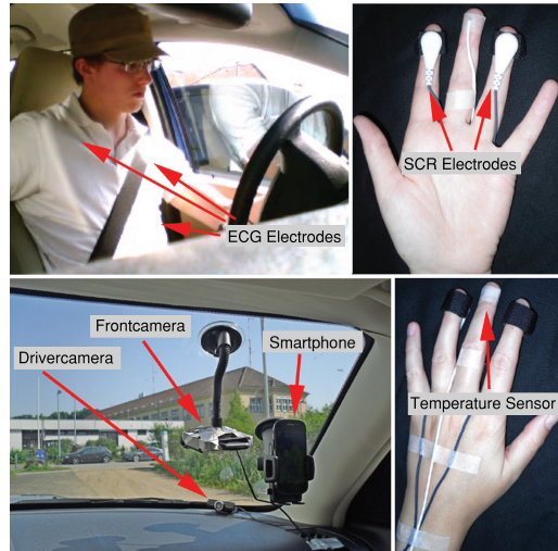
Figure 4.2: Apparatus for the real-world driving study: Two cameras and a smartphone are placed within the car (bottom left). Electrodes attached to the driver measure the ECG signal to extract heart rate and heart rate variability (top left). Skin conductance response (top right) and body temperature (bottom right) are measured at the drivers left hand.
