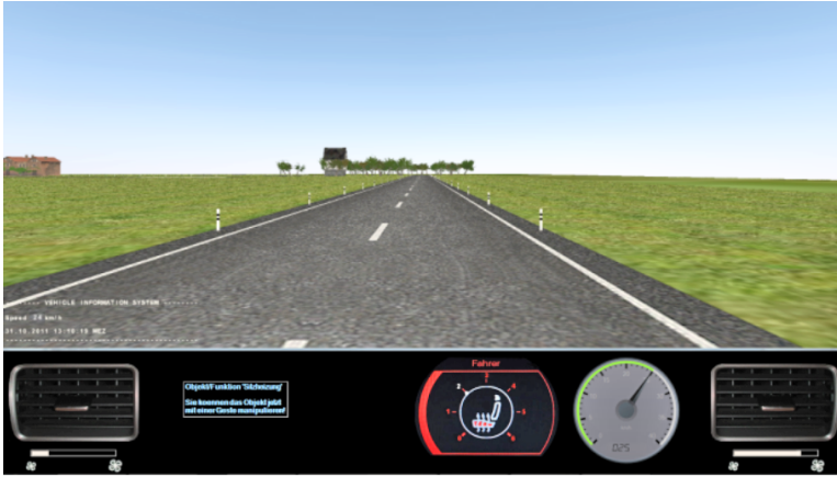
Figure 5.8: Screenshot of the driver’s view: Most part of the front TV screen is used to display the driving scene that is augmented with a rudimentary head-up display. The lower part shows the vehicle dashboard including visual representations of air vents, speedometer as well as an output space for additional visual feedback.
