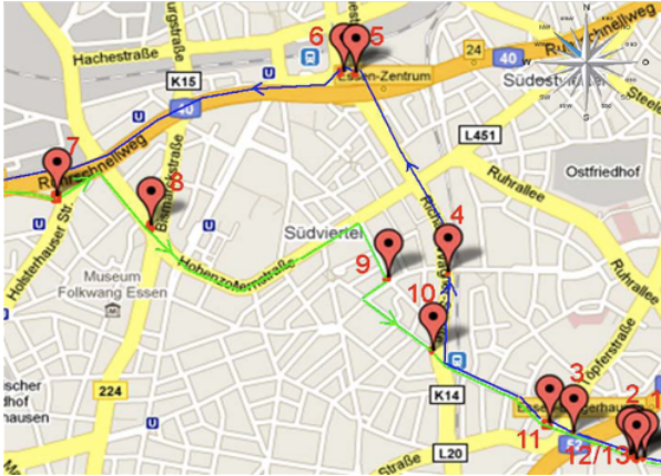
Figure 7.7: Evaluation route to test the concept of time-adjusted media with pre-recorded TLZs. The markers depict locations where the system detected the car as standing. Blue color is used to show the outward trip and green color for the return trip. Map data: Google, Tele Atlas.
