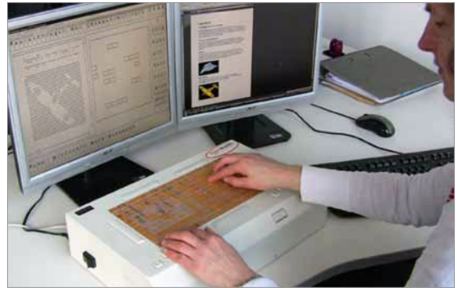
Fig. 9. HyperBraille device used to display graphical content [21].
