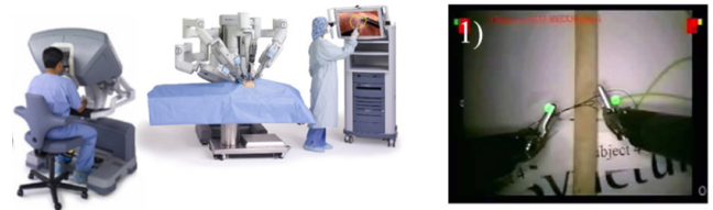
Fig. 15. Left: The Da Vinci Surgical System [10]. Right: Visible force feedback on a surgical robot [1].
