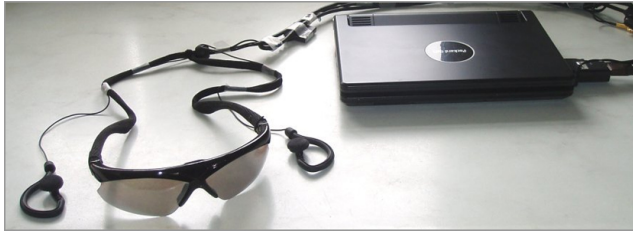
Fig. 7. The vOICe device consisting of a notebook, earphones and sunglasses including a camera [20].
