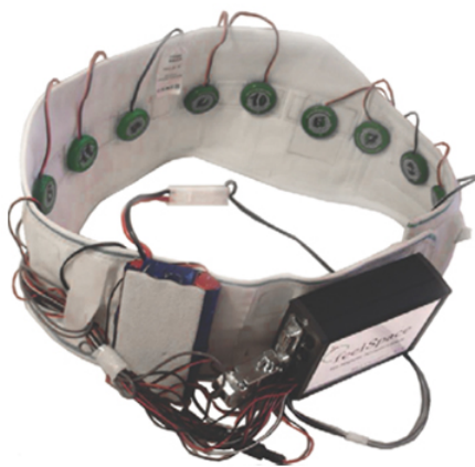
Fig. 14. Prototype of the FeelSpace belt with 13 vibrating motors [24]
