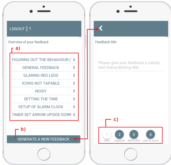
Figure 2. With CrowdUX users can provide feedback to products and services: left, (a) list of submitted feedback items, (b) button to create new feedback; right, dialog wizard guiding through feedback (c) title, capture (e.g., photo), description and rating.
