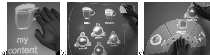
Fig.1. The mug metaphor interface. a) To move the mug/information container, the user touches its handle and drags it on the screen surface. b) To explore its content the user turns the mug. c) To cancel a unit of information, the user can drag it with the right hand to the drain displayed on the pie menu invoked with the left hand.
