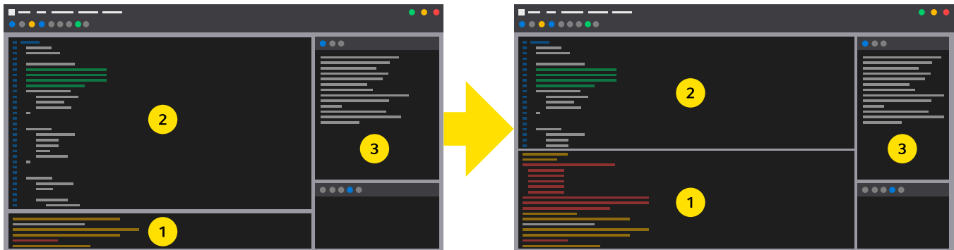
Figure 1: Our gaze-based adaptive IDE extension changes the layout of the IDE depending on the developers' intent. For example, when the prediction models determine an increased relevance for the terminal output in the IDE (1), the code editor (2) and other UI elements (3) shrink while the output panel (1) grows in size. This can highlight or reveal otherwise missed information.
