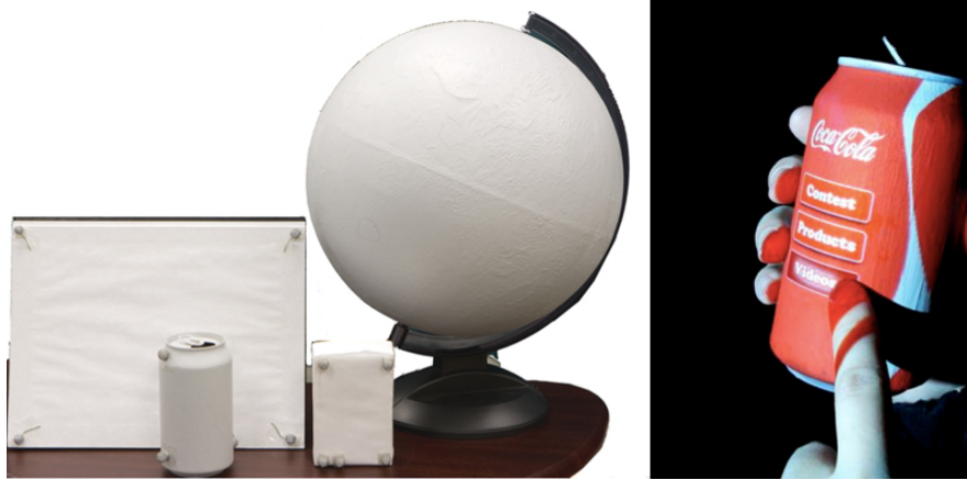
Figure 13. Mixed-fidelity prototyping, as practiced by Akaoka et al., using low-fidelity physical artifacts (left) and projected, digital artifacts (right), (Akaoka et al., 2010). 9
