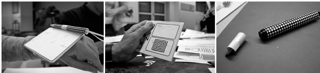
Figure 23. Initial ideas from a brainstorming session were rapidly turned into low-fidelity mockups representing different interaction opportunities: A wearable, GUI based device on the right, a NFC enabled device in the middle and an idea for using pointing as interaction mechanism with a removable data storage cap. 24
