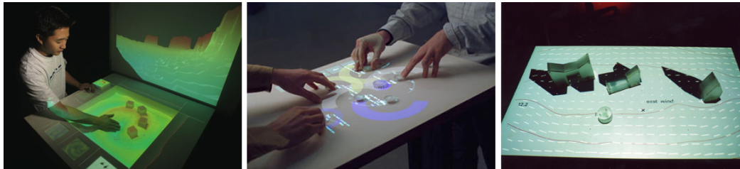
Figure 3. Use cases of TUIs in different contexts (from left): SandScapes (Ishii, 2008), a project to explore elevation levels physically, AudioPad (Patten et al., 2002), a musical device and the digital/physical work-bench URP, a tool intended to help city planners (Underkoffler and Ishii, 1999). 2
