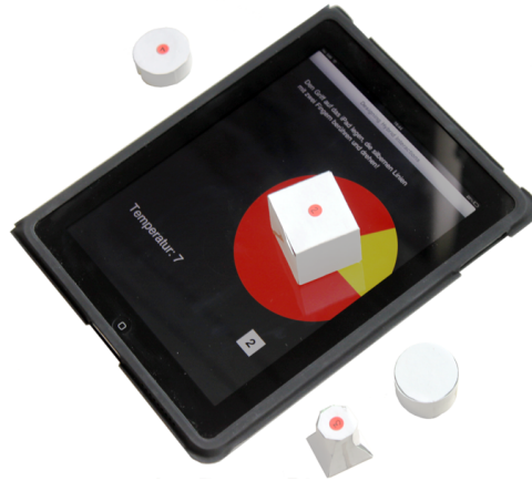
Figure 40. A working Sketch-A-TUI prototype showing the graphics it is controlling on an iPad (Wiethoff et al., 2012). 41
