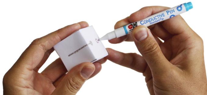
Figure 36. Sketching conductive ink on a cardboard object creates a tangible object recognized by a capacitive surface (Wiethoff et al., 2012). 39
