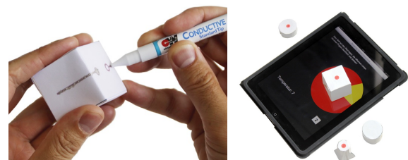
Fig. 4 Sketching conductive ink on a Paperbox object (left), and then using it to interact with a tablet (right) [19].
