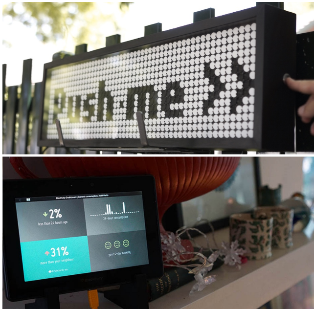
Figure 3. The Flip-Dot display with the push-button located on its side for triggering a data-driven short animation (top), and the tablet app to control the content on the low-res display (bottom).
